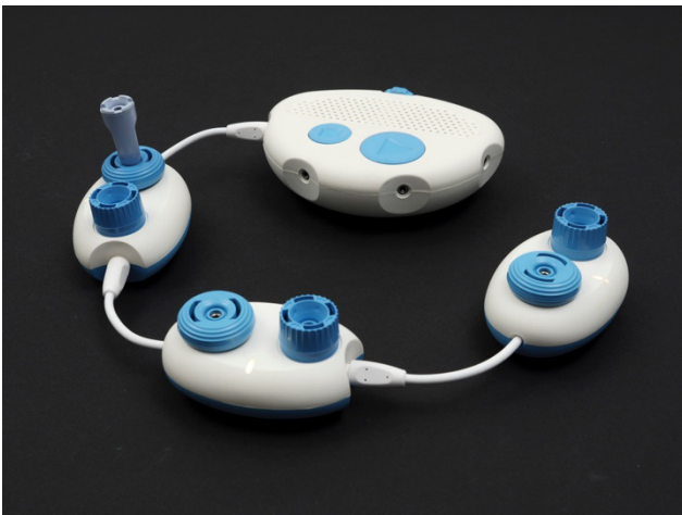
[Figure Caption:] This photo shows a Code Jumper program with three Play pods connected, one after the other, to the Hub at Port 1. A Variable plug is connected to the port on the first Play pod’s Sound dial.
